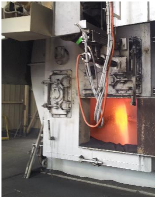
Infrared camera PYROINC 380LF with air purge, water cooling and emergency retraction
