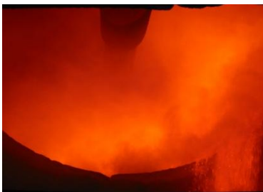
CCTV-Image: view through the kiln very poor due to high dust concentration.
