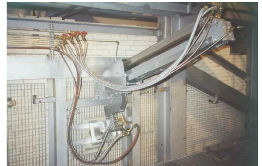
Infrared camera PYROINC 768N with air purge, water cooling and emergency retraction device
